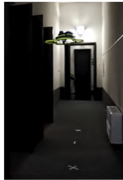
Figure 2 Autonomous indoor flight through a corridor during testing. The drone adapts to tight spaces using onboard SLAM and visual cues.
