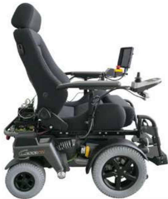
Figure 1: The wheelchairs designed in the project and operated using the methods described here were equipped with depth imaging cameras, laser scanners (at the front and the back of wheelchair, not visible here), odometers, user interfaces, and a computing unit.
