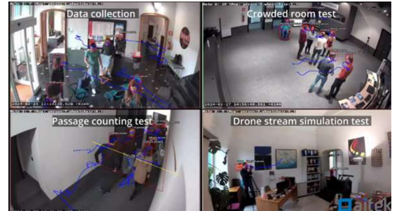
Figure 1 - Examples of framing and event detection through the smart monitoring system.
