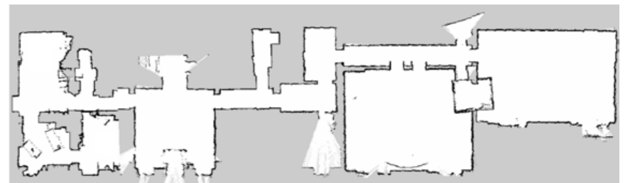
Figure 4 Map of the CNR generated by fusing the wheelchair's and the drone's maps
